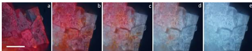
Figure 23. Optical micrographs of KCAT crystals exposed to H 2 gas for a) 0 min., b) 55 min., c) 85 min., d) 112 min., e) 150 min. Scale bar = 100 \mu m.
